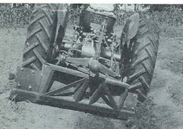
Shallow or Deep Ditching . . . Matched to a Ferguson System Tractor for deeper ditching and excavating. Correct moldboard curvature rolls the dirt, moves more dirt with less power.
