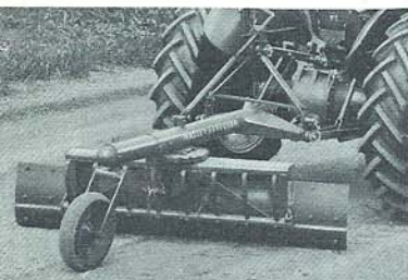
Smooth, Even Grading . . . Builds and maintains dirt or graveled roads same way costlier graders would. Keeps farm roads and rutted lanes open at low cost.
